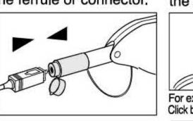
Remove your ferrule or connector from the Ferrule guide and close the Tip cover of the Protection cap.
