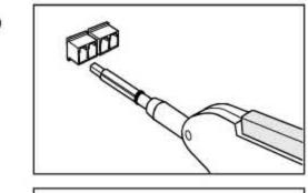
Push in until Stopper of Cleaning guide comes in contact with the adapter.
