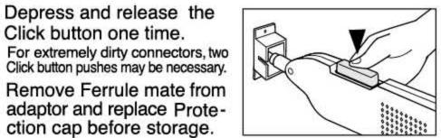
Depress and release the Click button one time. For extremely dirty connectors, two Click button pushes may be necessary. Remove Ferrule mate from adaptor and replace Prote-
